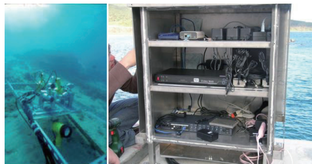
Figure 6. Illustration of the underwater video cameras and the video server
