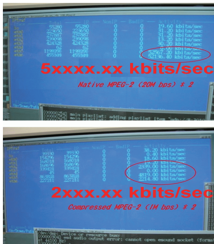
Figure 4. Illustration of the bandwidth with/without distributed stream compression concepts.
