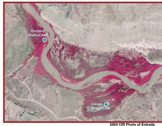
Figure 2. We set up infrastructure for long-term monitoring of ET using point measurements from sap flux sensors, percent cover from “PhenoCAMS” and scaling ET to the river reach / landscape scale using imagery (ASTER and MODIS).
